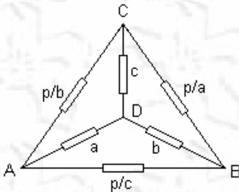
$$R_{AB} = \frac{ab + ac + bc}{c} = \frac{p (\Omega^2)}{c (\Omega)}$$
